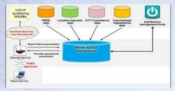
Figure 1: Typical implementation of Geolocation Database based TVWS technology
